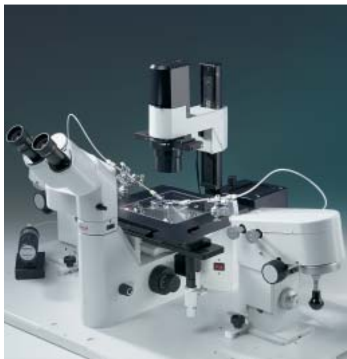
Leica Micromanipulators with the Leica DM IL microscope for examination of cell and tissue cultures
