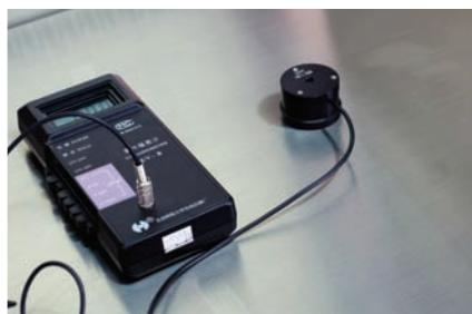
Integrity testing of HEPA filters
