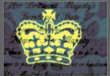
UV fluorescent security feature is revealed using UV 365nm illumination.
