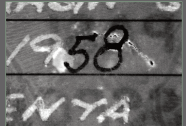
IR fluorescence examination reveals the presence of two different inks
