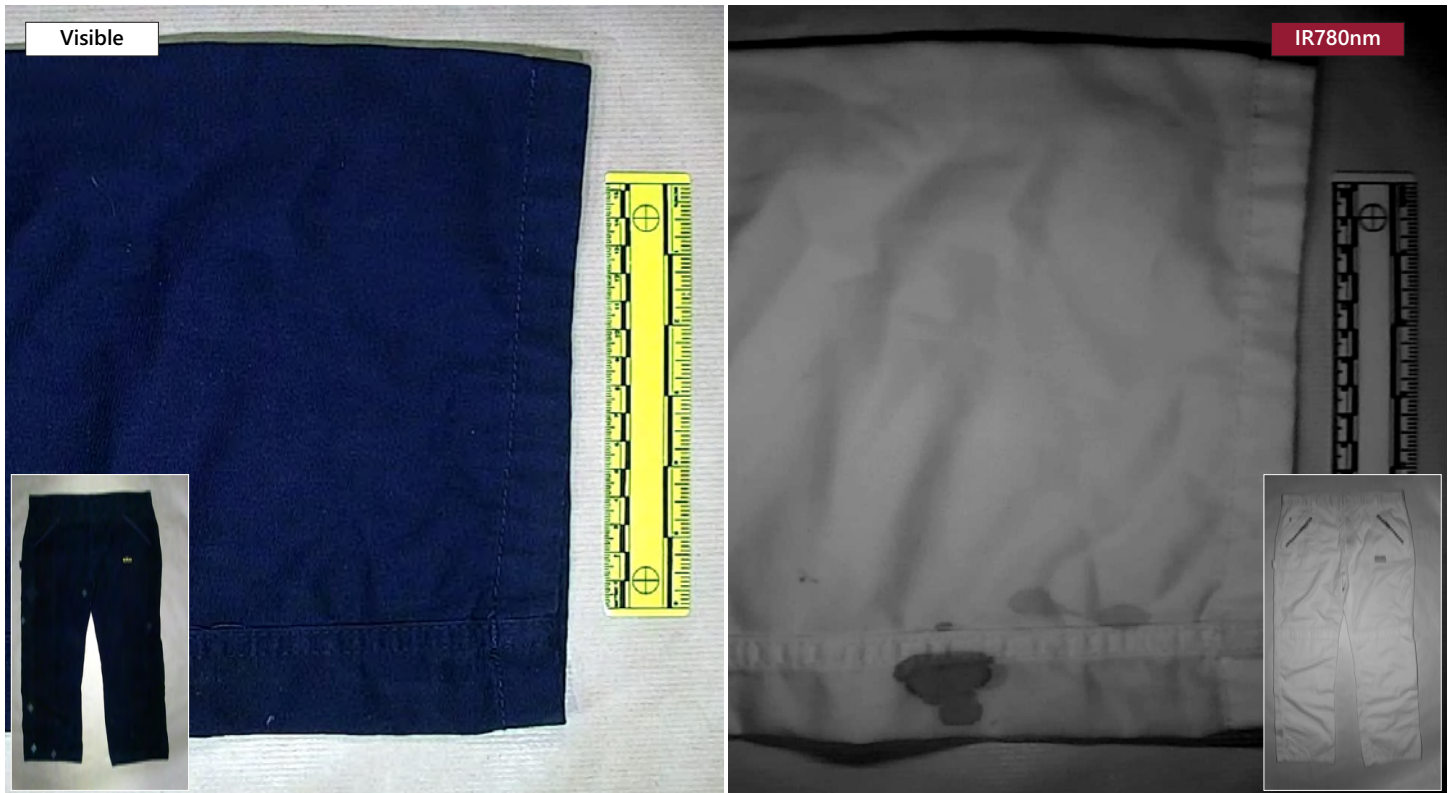
Blood is visualised on dark material using IR 780nm illumination. The material 'drops out' while the blood absorbs the IR
